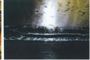
Figure 16: Crack through the weld
